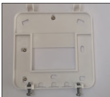
Fix the backplate to the wall
